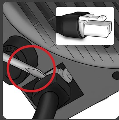
**Removing the White Connector from the Power Supply Unit:**
