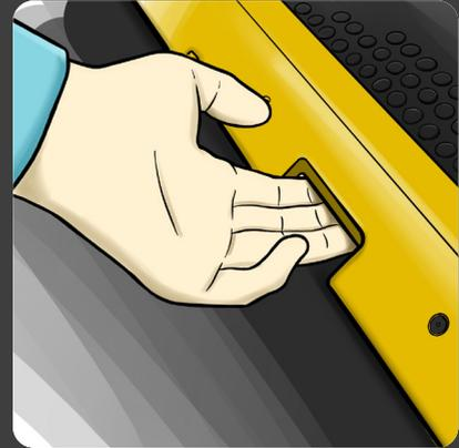
6) To lift the mat, place 2-3 fingers under the central slot on the metalwork edge and lift upwards.
