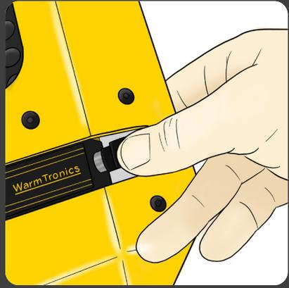
**Removing the Black Connector from the Heat Mat:** To disconnect the cable from the heat mat, the black end has a spring to pull back and release the connector.
