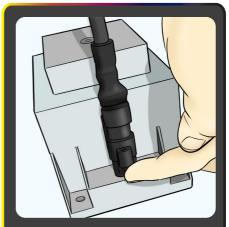
Disconnecting the Power Supply Unit: Turn off at the mains plug and unplug, then push the pin on the Power Supply Unit connector to 'unclick' it. Do not lift up the Power Supply Unit by the power cable.
