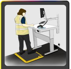
5) Stand on the mat. To switch the heat off, press the button until a single blue light remains. When not in use, switch off at the mains socket.
