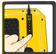
4) Press once for low heat, twice for medium heat, and three times for high heat.
